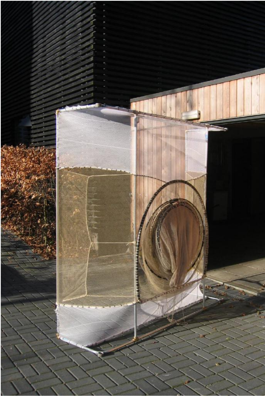
Fyke net construction for fish pass monitoring at Wier.
